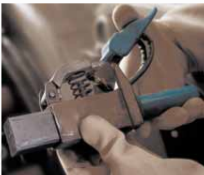
Changing and checking of the brush are carried out in safety - outside of the running motor.
